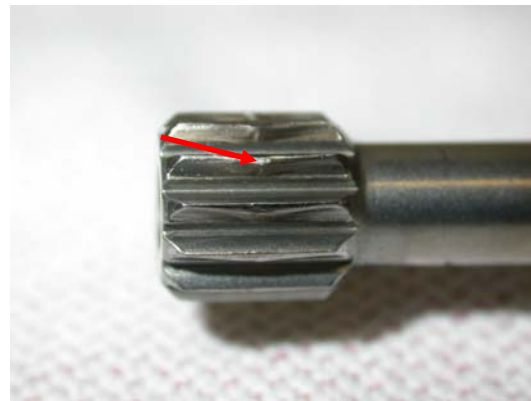
Fig. 6 Wear on control drive shaft spline
