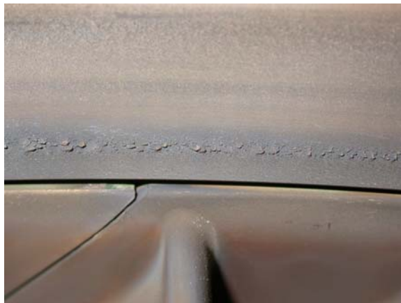
Fig. 7 HPT STG 1 Shroud with build up material
