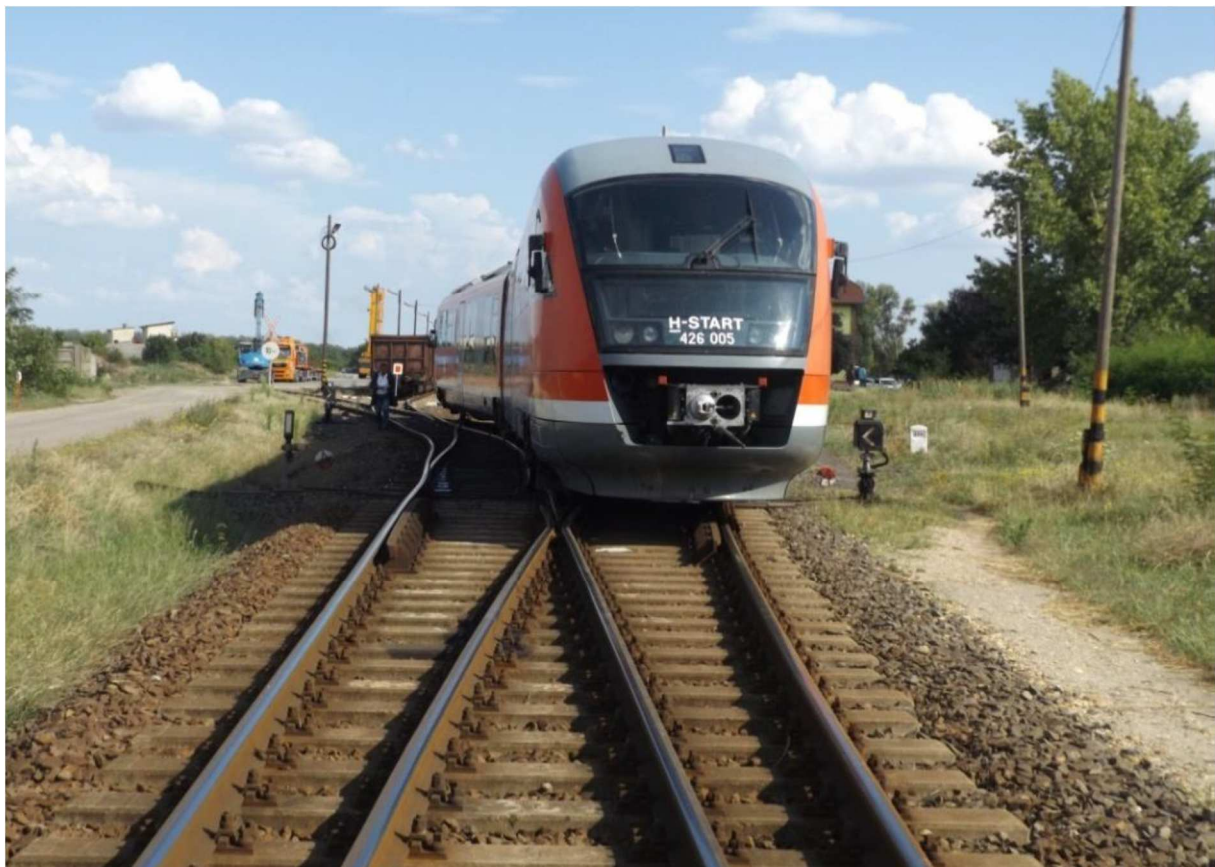
Figure: The derailed motor train set
