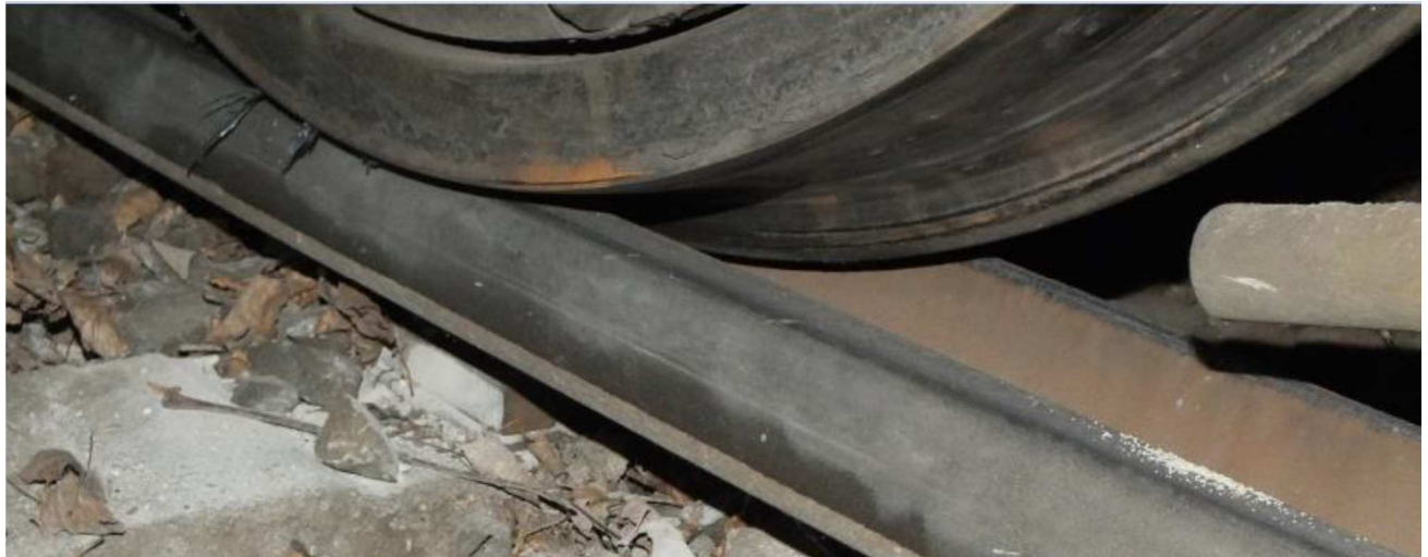
Figure: A wheel of the derailed vehicle on the rail which had tipped to its side
