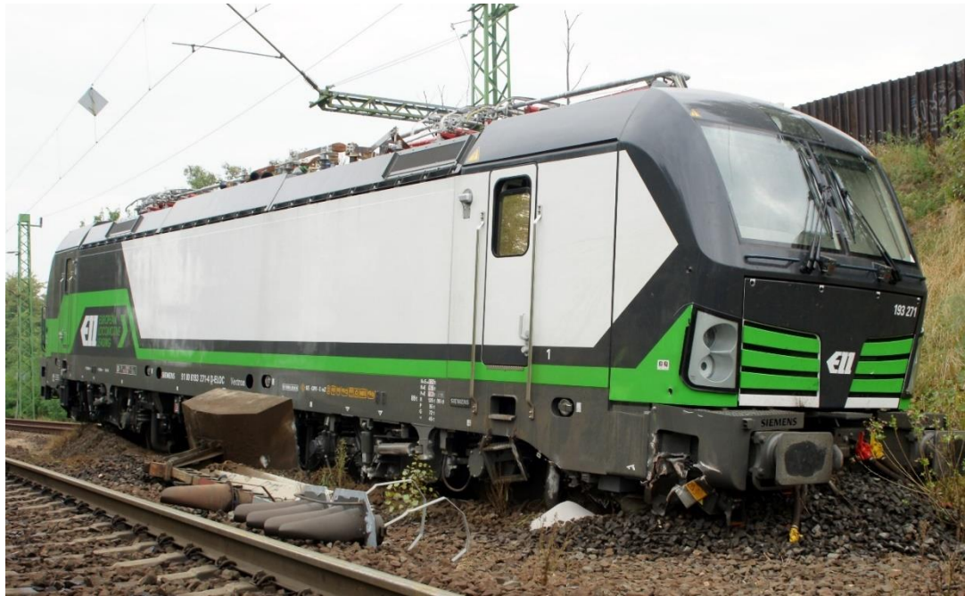
Figure: The locomotive hit the earth pile and derailed
