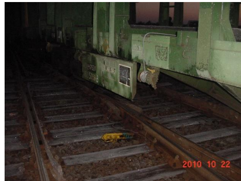
Picture 2: Drag shoe found on the site (source: VBO)
