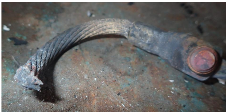
Appendix 3: Melted surface of the electrical cable
