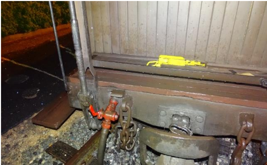
Figure 4: The brake spindle and a rail skid on the passenger wagon with reg. № 305
