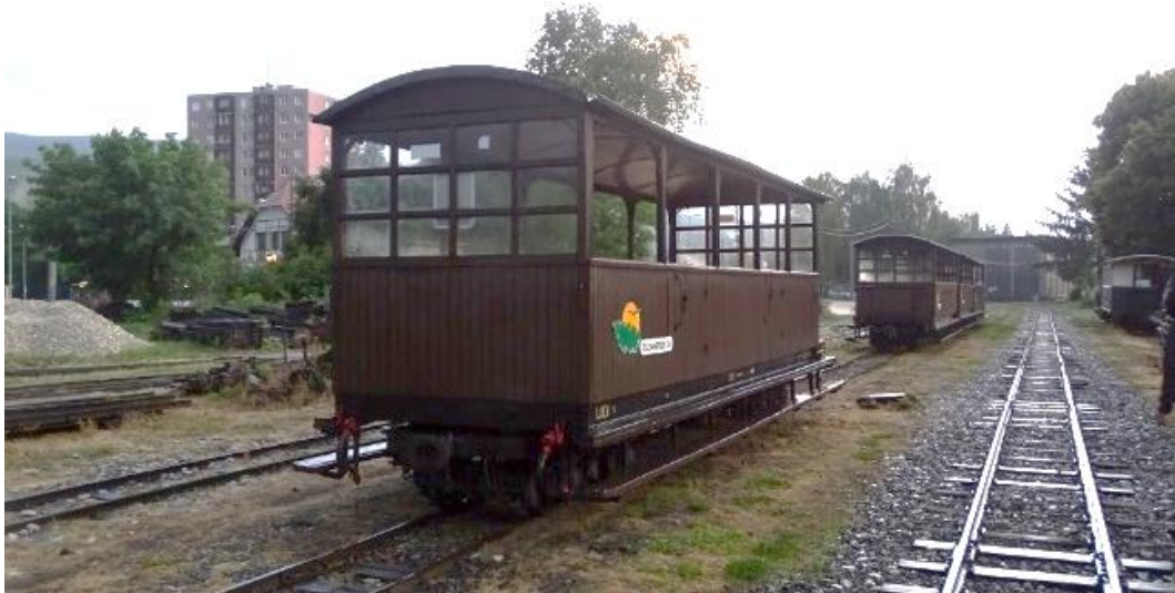
Figure 6: Wagons stopped without any rail skids applied on Track III at Majláth Station
