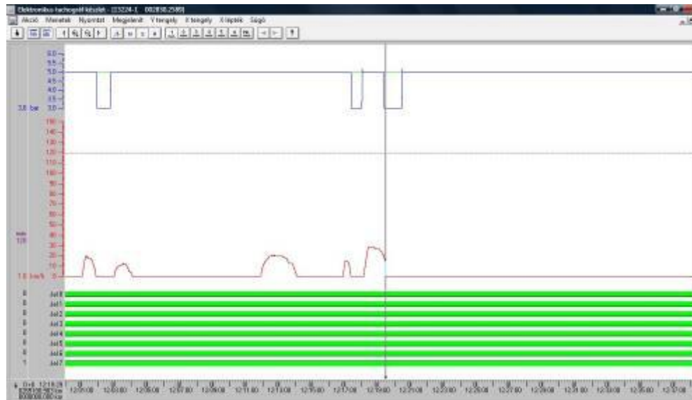
Figure 6: strip chart recorder of V43-3313 locomotive
