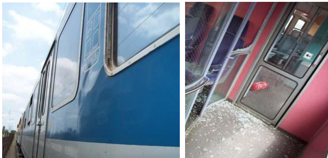
Figure 4: external and internal damage of the carriages
