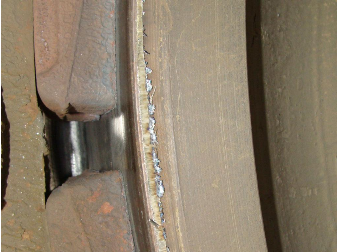
Figure 4: marks (scrapes) on the wheel of the locomotive
