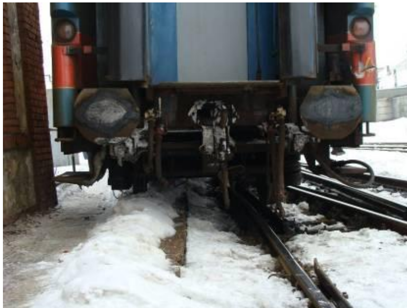
Figure 3: the derailed carriage beside the wall of the points operation building
