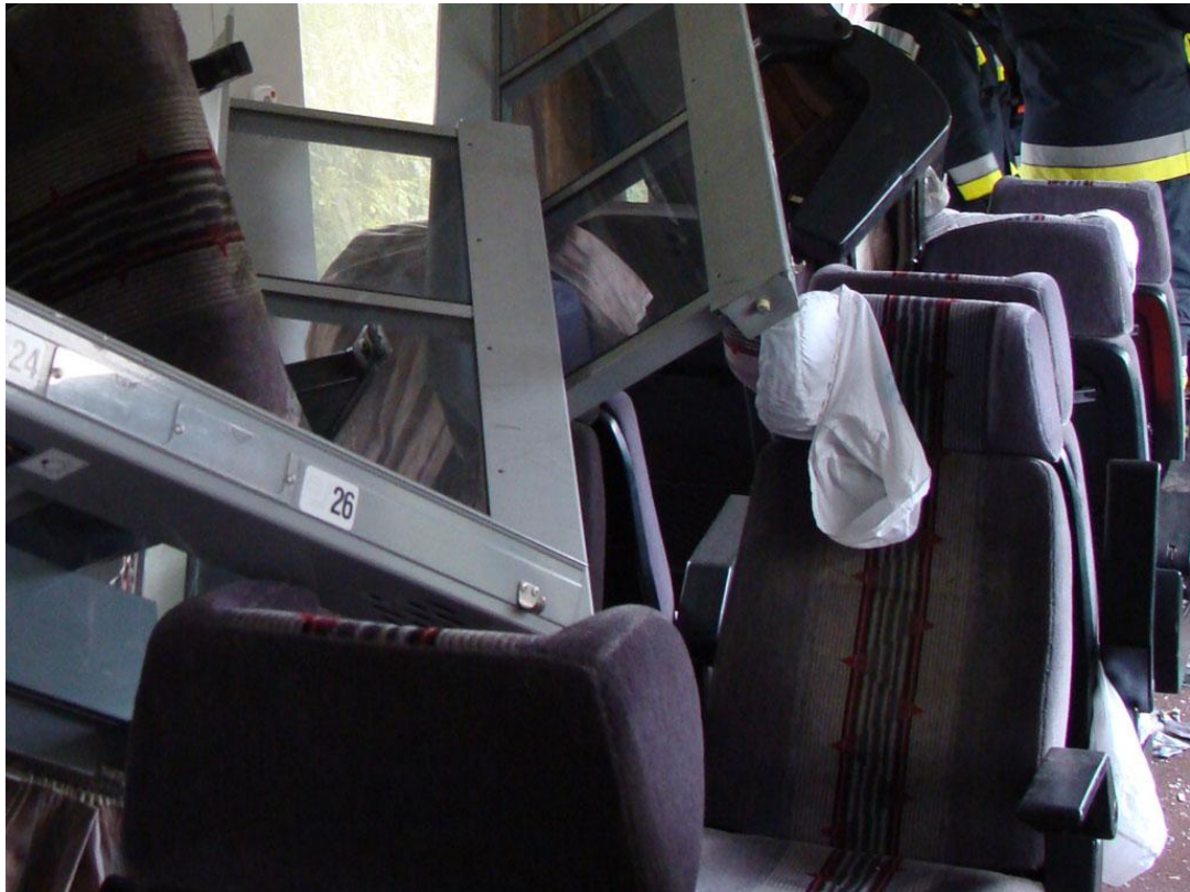
Figure 24: Torn down, broken luggage racks in between and on top of the seats
