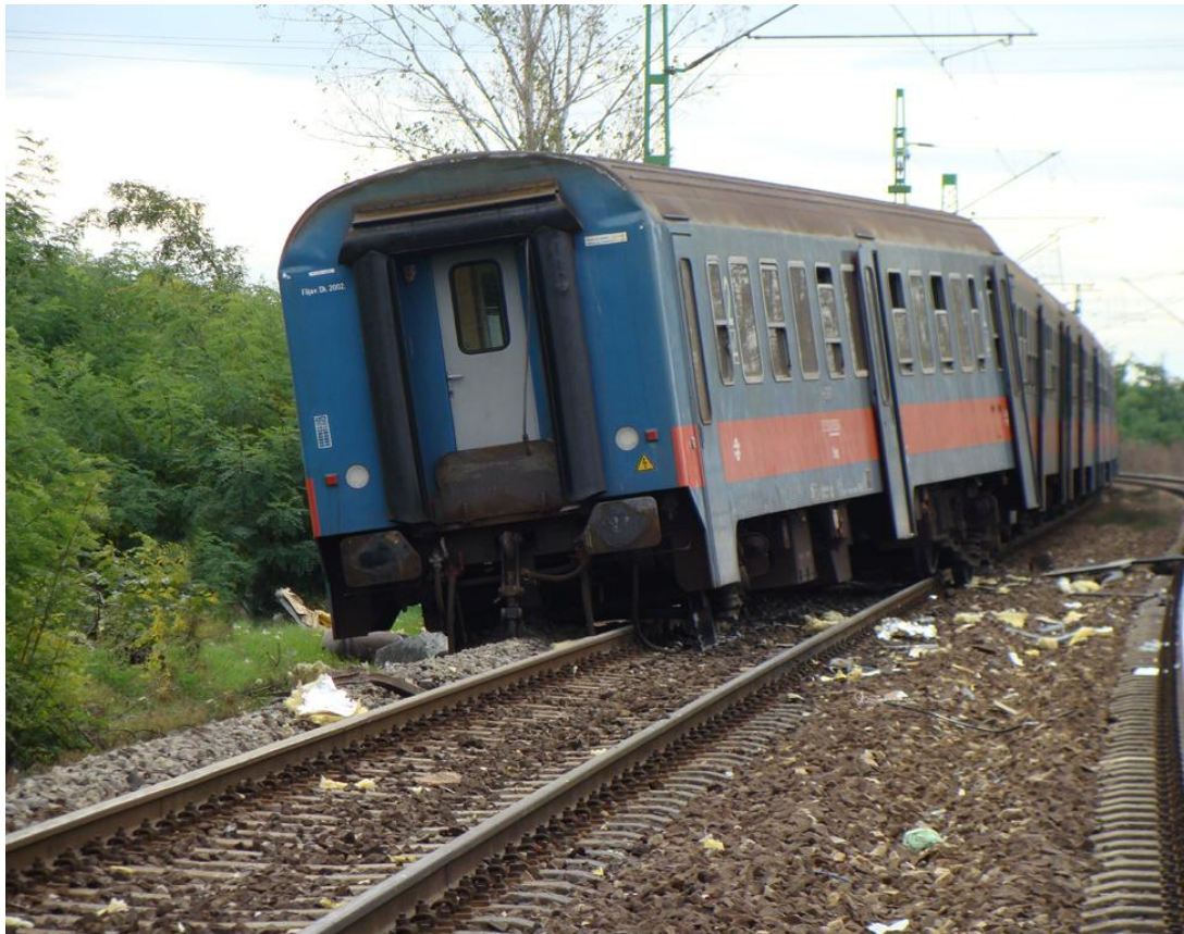
Figure 6: The derailed second carriage of the passenger train and some scattered debris
