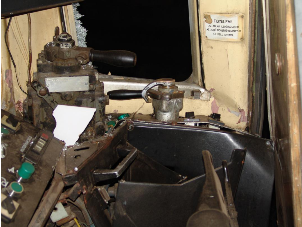
Figure 11: The driver's cab of Bzmot 212 motor coach after the collision
