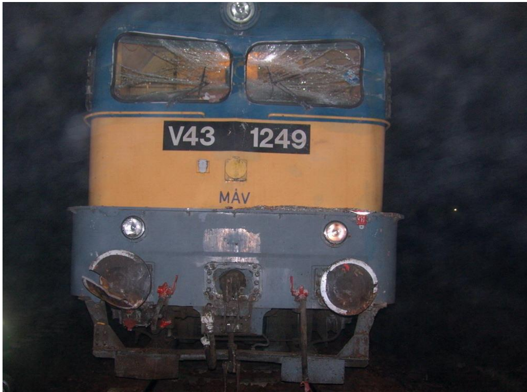
Figure 10: Locomotive no. V43-1249 after the collision
