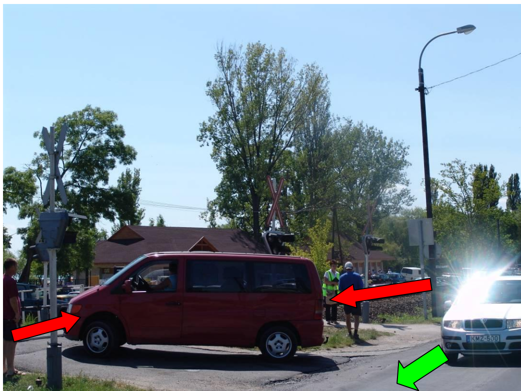
Figure 25: Running trains may reach and collide with vehicles passing the warning lights or those stopping in the clearance
