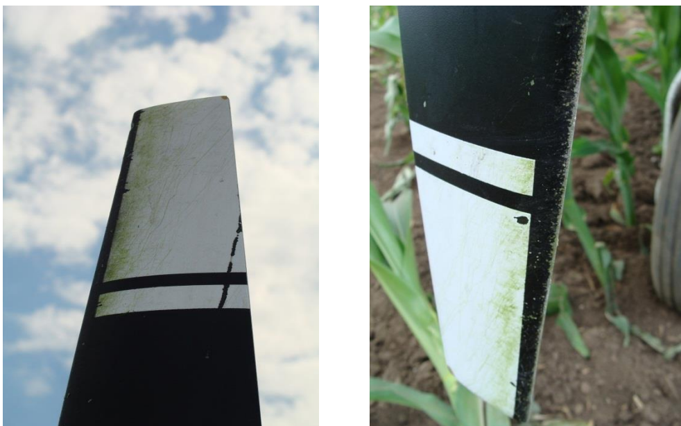
Pictures 3 & 4: Marks from the vegetation on the outer sections of the propeller blades after the aircraft landed and stopped
