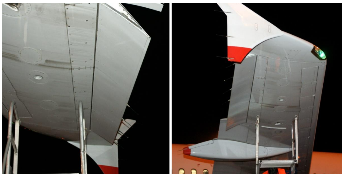
Figures 2 and 3: Position of the right aileron with pressurized hydraulic systems after landing
