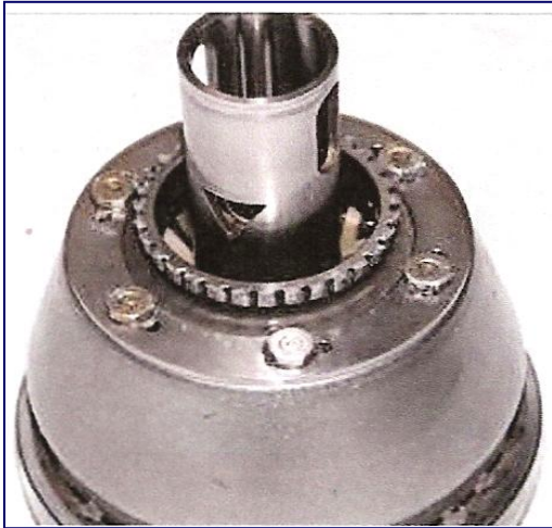
Fig. 1. The worn gear ring
