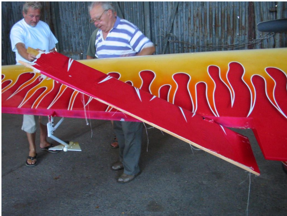
The left wing and the remains of the aileron
