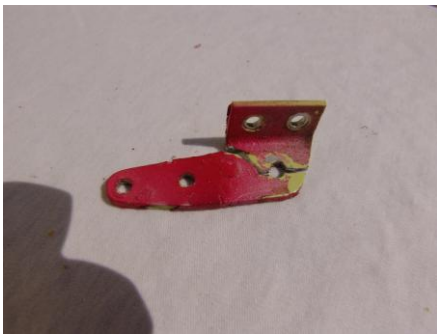
Bracket right eyelet fracture
