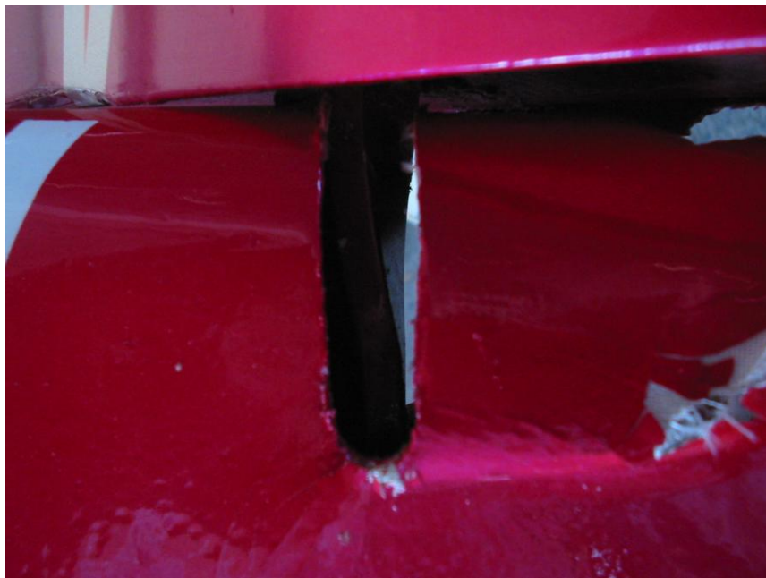
Damaged inner hinge
