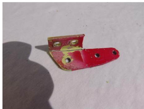
Bracket left eyelet fracture at its base
