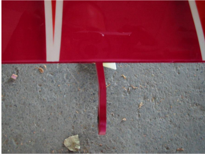
Damaged center hinge
