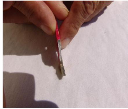
Grainy structure (dynamic fracture)
