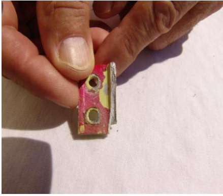
Fracture surface of left eyelet
