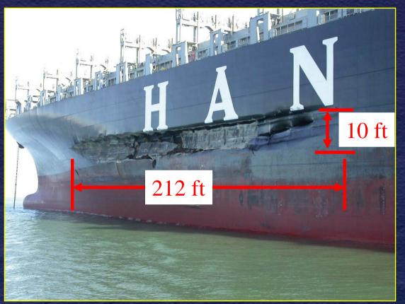
Damage: \$2.1 M Size: 220 ft x 14 ft Spilled: 53,500 gal
