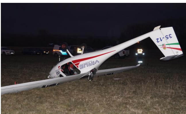
Figure 2. - The aircraft on its back with bent spoilers
