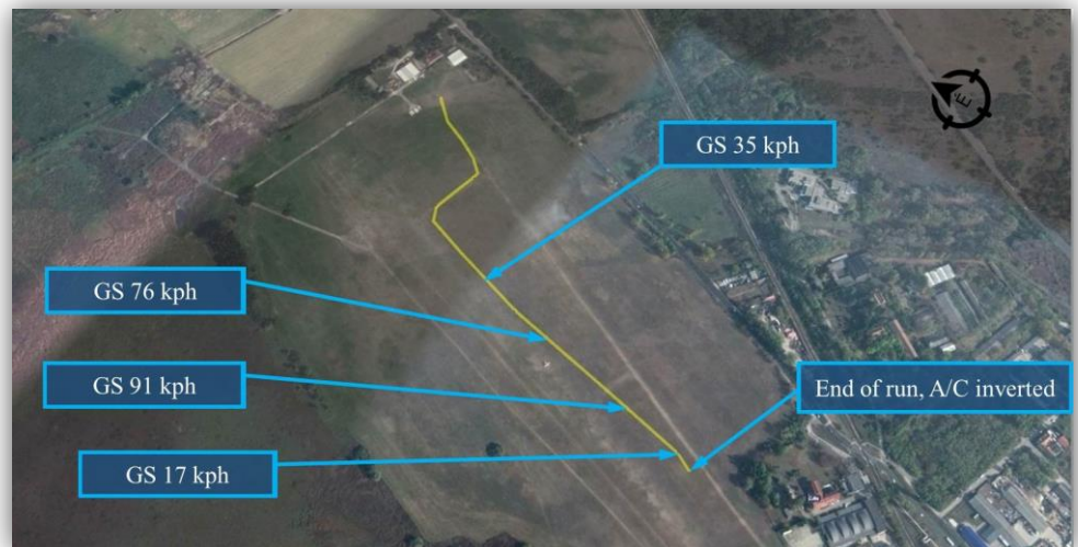
Figure 1. - Acceleration track and speeds as recorded by the on-board GPS (GS: ground speed, 'É' represents North in the compass rose)
