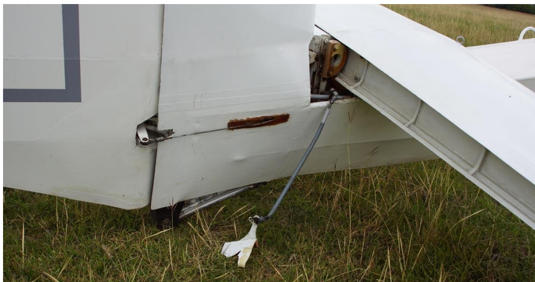
Figure 4: The RH horizontal stabilizer. Note the trim linkage with a piece of trim
