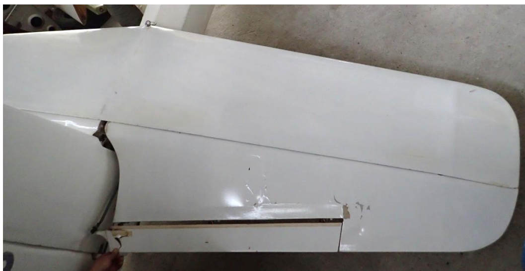
Figure 10: The RH elevator re-attached to the horizontal stabilizer
