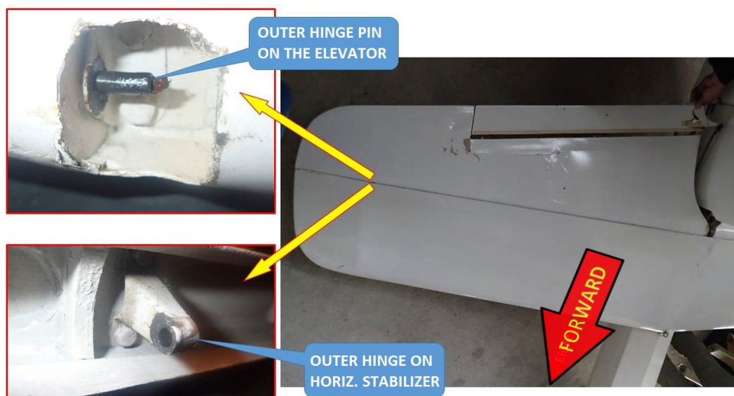
Figure 9: Top view of the RH elevator with fixing locations
