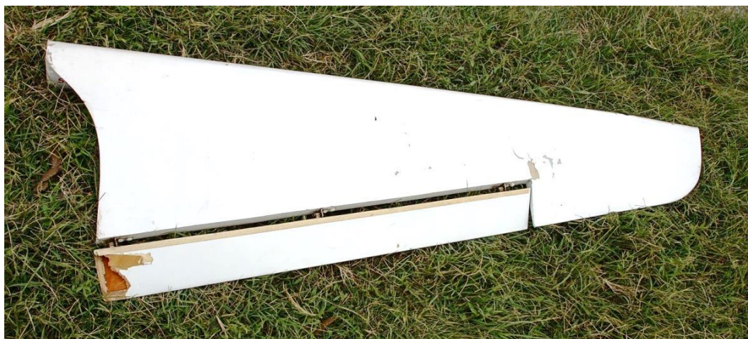
Figure 5: The damaged RH elevator and attached trim
