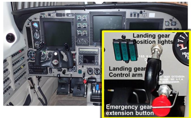
Figure 4 – Landing gear controls in the cockpit
