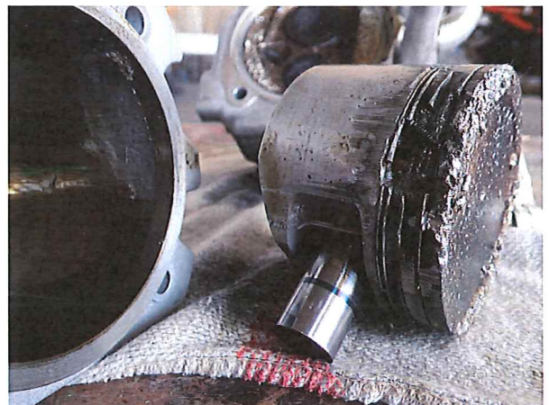
Figure 2: The damaged piston
