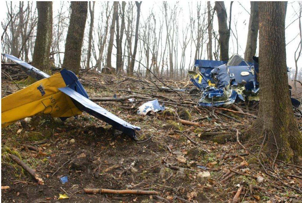
Figure 7: The wreck of the aircraft with some major structural elements separated (Photo: TSB)
