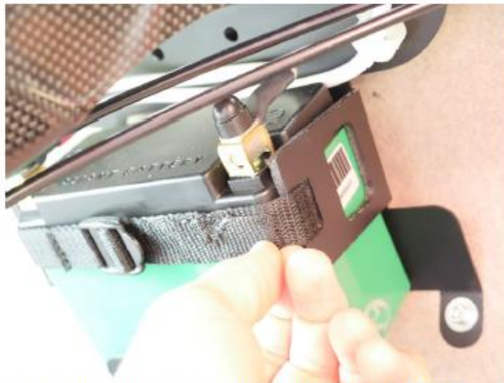
Figure 2: Fore battery installation – tearing away the strap's loose end
