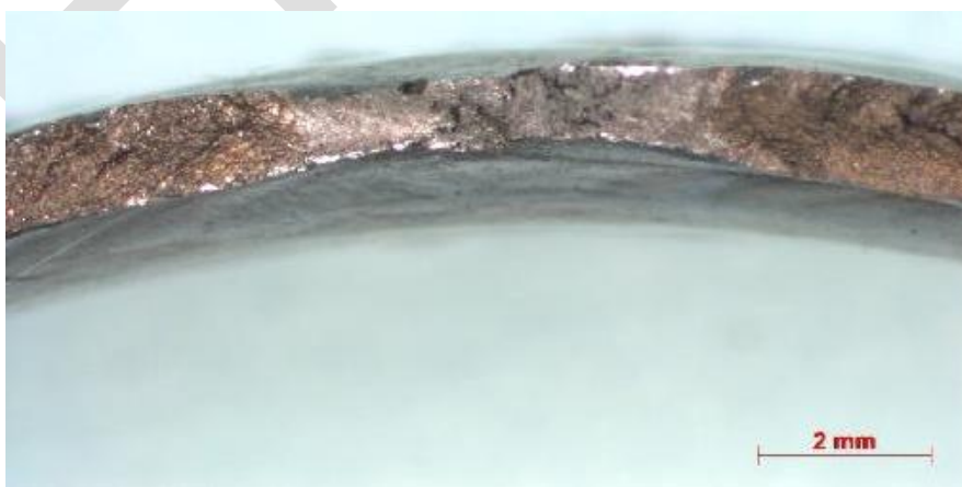
Figure 9: Evidence of the cracked surface of the pipeline caused by fatigue
