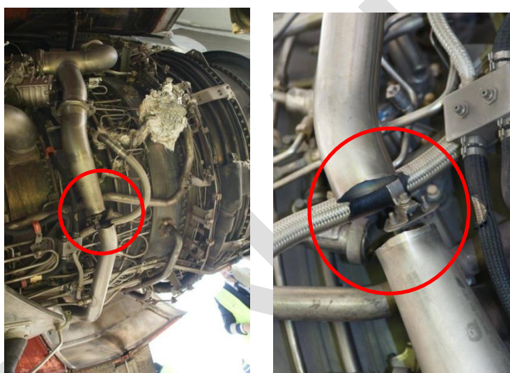
Figure 8: The broken pipeline in the installation area
