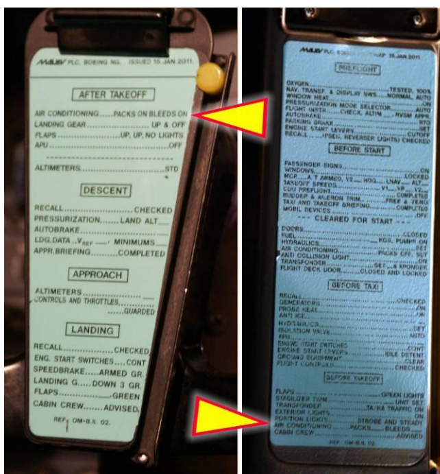
„Normal” checklists displayed in the cockpit (the line relevant to air conditioning are indicated in the before and after takeoff checklists)
