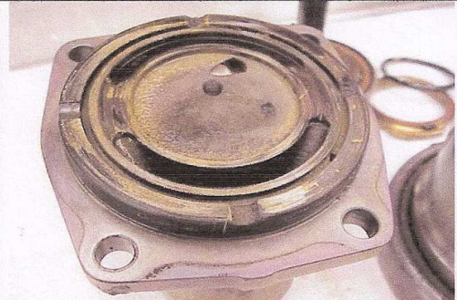
Pump – Port Cap with bronze material transferred
