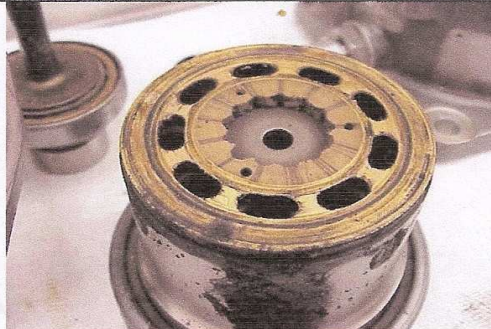
Pump – Cyl. Barrel face worn
