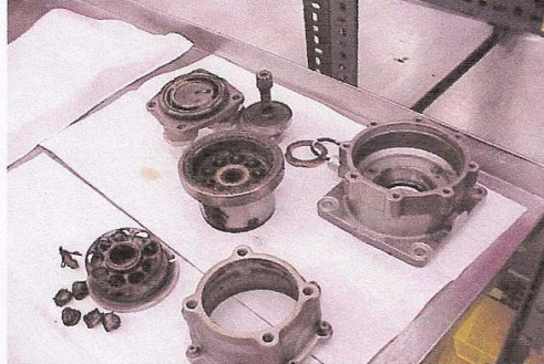
Pump side components – overheated, and damaged
