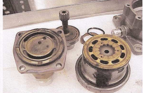
Pump – Port Cap & Cyl. Barrel face heavy galling
