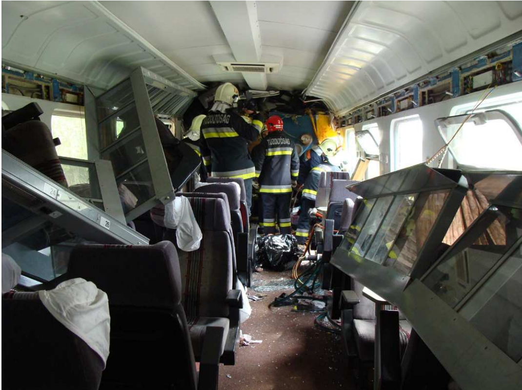
Figure 5: The inside of the last carriage of train no. IC 560-1 with the torn off luggage-racks
