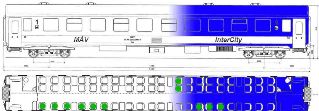
Figure 11: The last carriage of train IC 560-1; the destroyed part of the passenger compartment indicated with blue and the sold seat tickets are indicated with green colour
