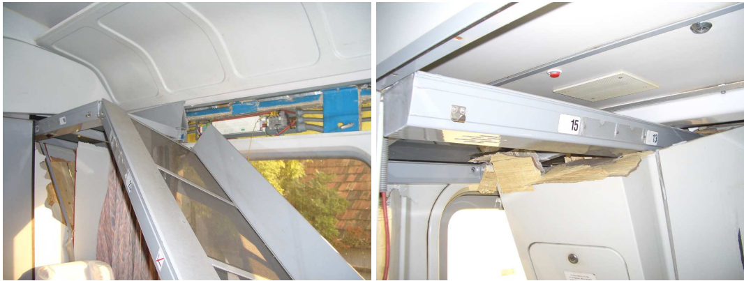
Figure 25: the luggage rack penetrating the wall of the toilet
