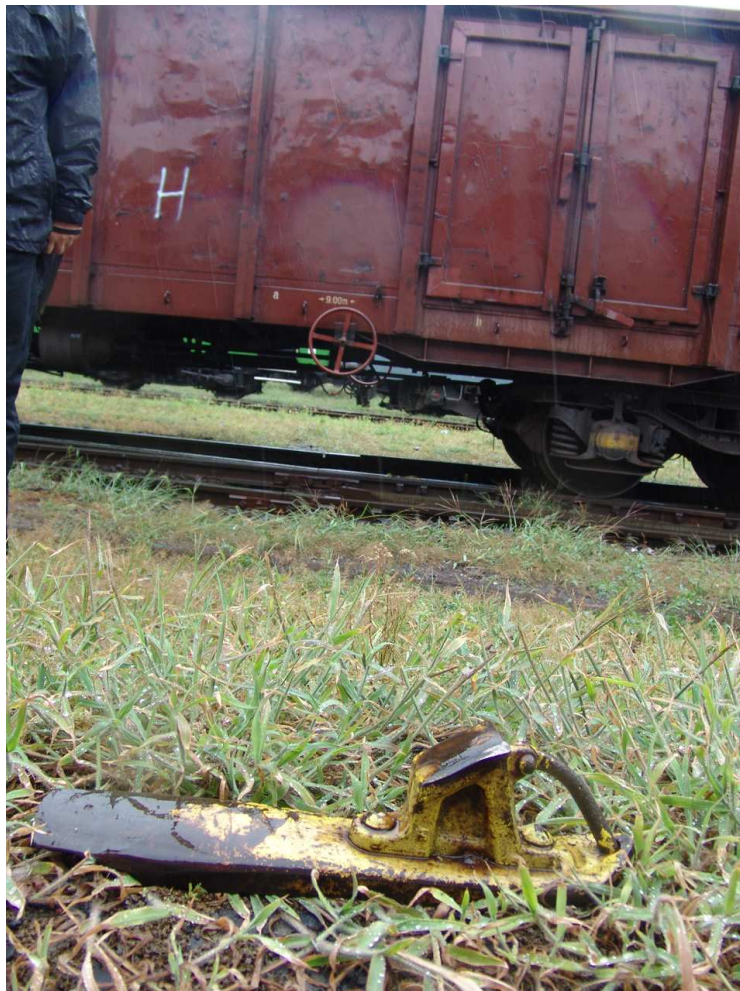
Figure 8: The scotch block left under the first freight car causing the accident.
